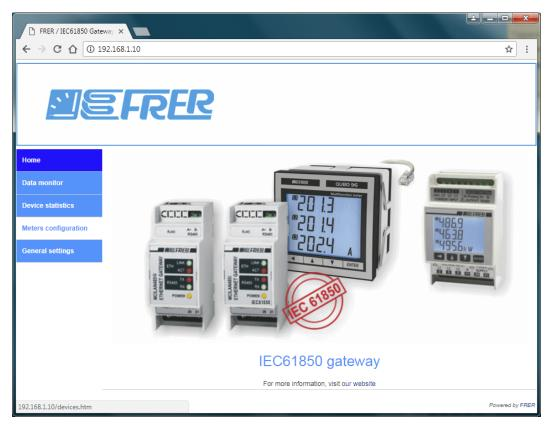
b) Press the "Meters configuration" menu item, and enter the credentials in the following login panel:
