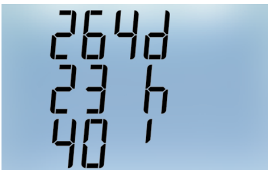
Hours run Value resettable by holding down the ◀ key at least per 3 seconds.
