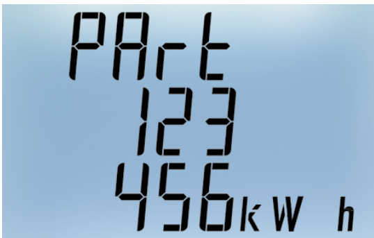
Partial consumed system active energy (Single Number expressed on 3 lines. In the example shown, the count corresponds to 12345678.90kWh) Value resettable by holding down the ◀ key at least per 3 seconds.
