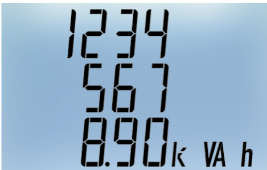
Apparent energy (Single Number expressed on 3 lines. In the example shown, the count corresponds to 12345678.90kVAh)
