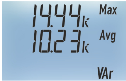
Average ractive power and maximum demand (kVAr) Moving average in a selectable time (see meter setting procedure)
