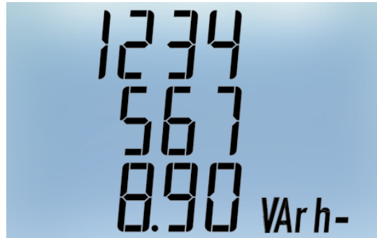
Generated system reactive energy (Single Number expressed on 3 lines. In the example shown, the count corresponds to 12345678.90kVarh)
