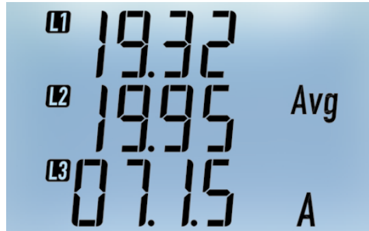
Average currents Moving average in a selectable time (see meter setting procedure)
