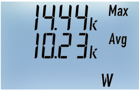
Average active power and maximum demand (kW) Moving average in a selectable time (see meter setting procedure)
