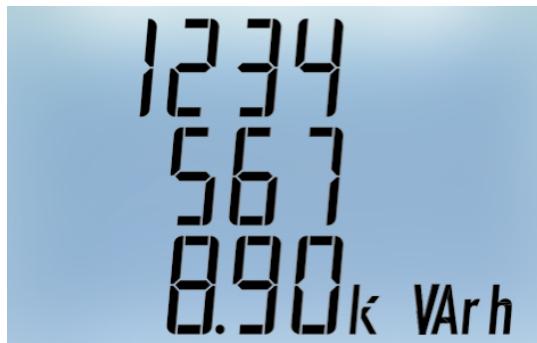
Consumed system reactive energy (Single Number expressed on 3 lines. In the example shown, the count corresponds to 12345678.90kVarh)
