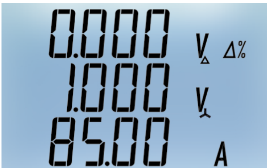
Unbalance phase delta voltages and phase currents
