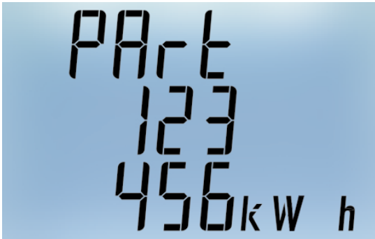
Partial consumed system active energy (Single Number expressed on 3 lines. In the example shown, the count corresponds to 123456kWh) Value resettable by holding down the ◀ key at least per 3 seconds.
