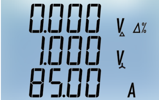
Unbalance phase delta voltages and phase currents
